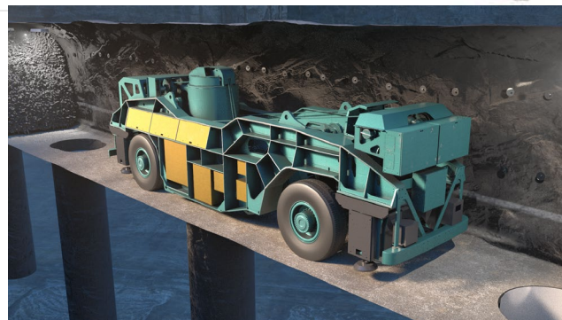
Canister installation machine
