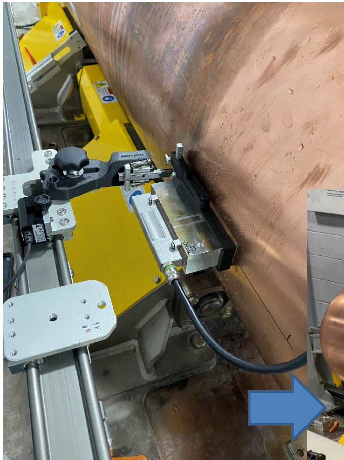
Copper Inspection (NDE)
