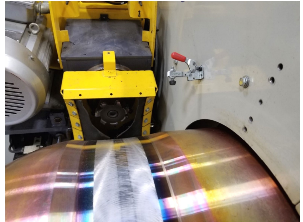
Weld Cap Machining and Inspection (NDE)
