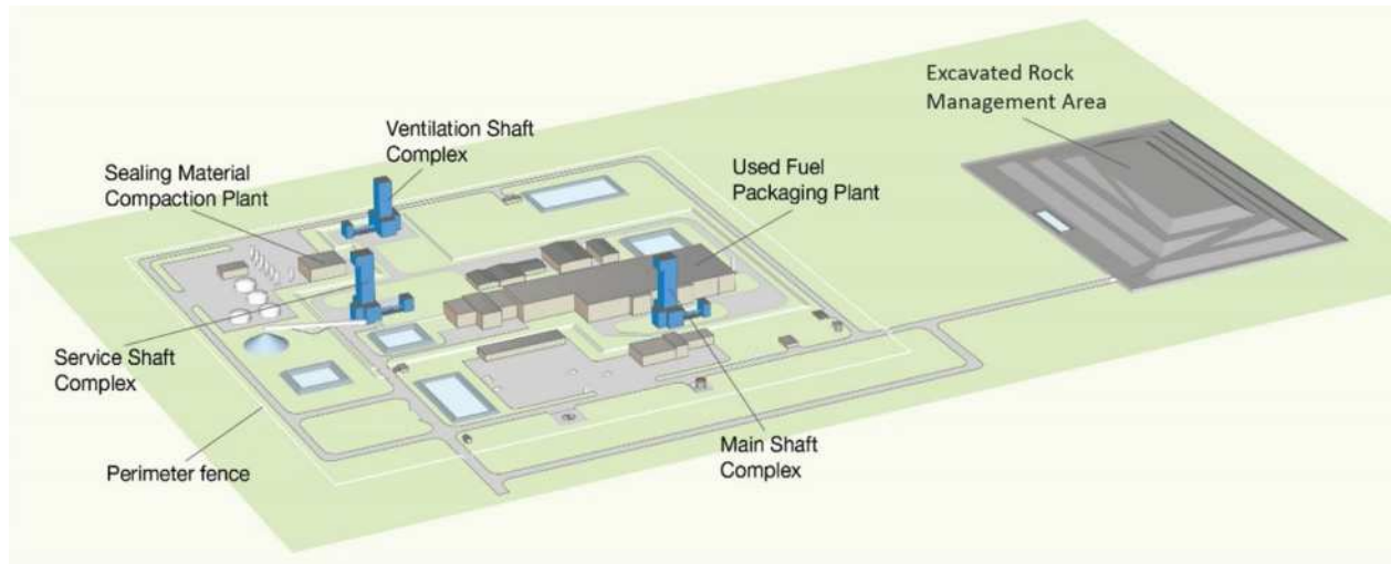
Figure 4-2 Conceptual Illustration of Surface Facilities (NWMO 2021d)
