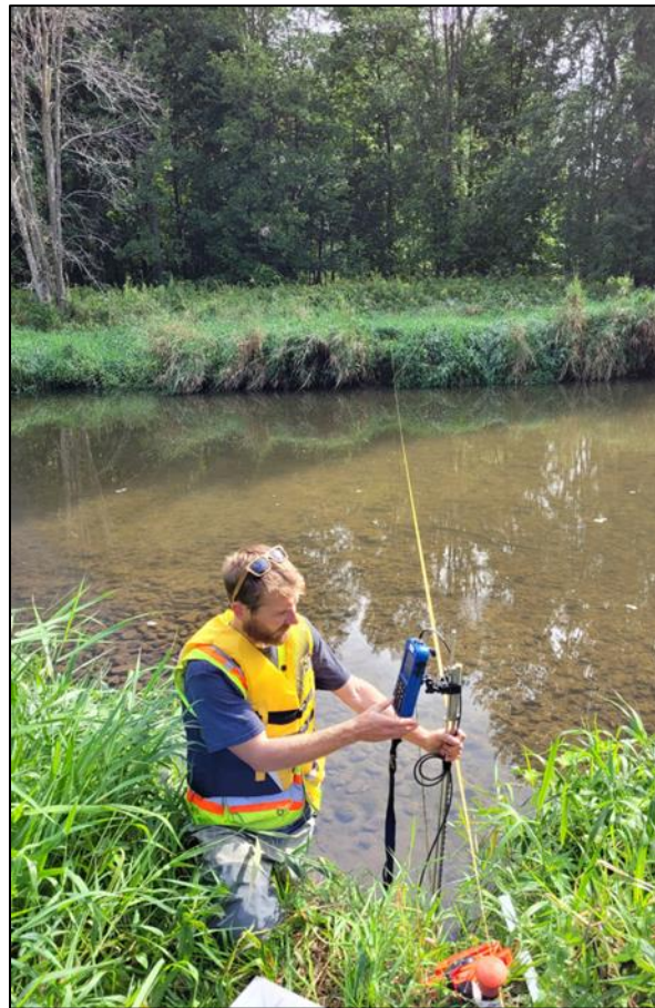
Figure 5. SVCA personnel collecting flow and depth data in the Teeswater River using an OTT MF Pro water flow meter.
